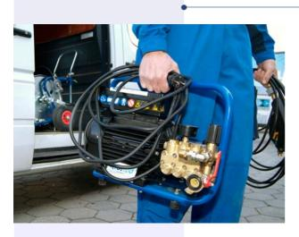
The MiniJet is a professional high pressure jetting machine, that can be taken everywhere without problems. It is suitable to clean drains from 25 – 100 mm.
