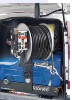
The CityJet can carry more water without compromising on space, due to the new design of 2 separate Rioned Compact System® water tanks, making the handling of the vehicle much smoother.
